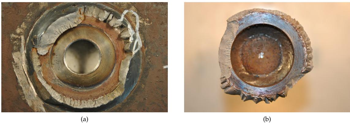
Figure 41: Fractured surfaces from torsional loading: plate view (a) and pipe view (b)
