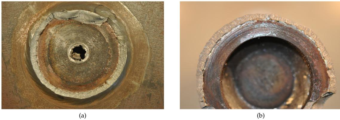
Figure 42: Fractured surfaces from bending loading: plate view (a) and pipe view (b)
