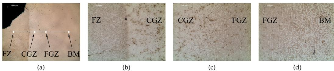
Figure 38: Optical microscope micrograph of the joint in AW condition. Focus on the weld toe showing FZ, CGZ, FGZ and BM (a). Detail of the microstructure transition between FZ and CGZ (b), CGZ and FGZ (c), FGZ and BM (d)
