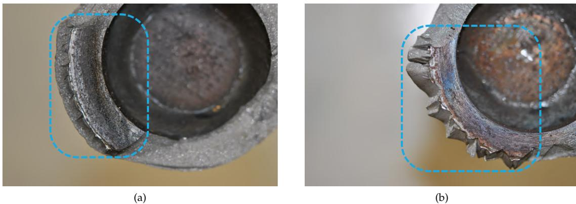
Figure 43: Fractured surfaces for pure bending (a) and pure torsion (b) loading
