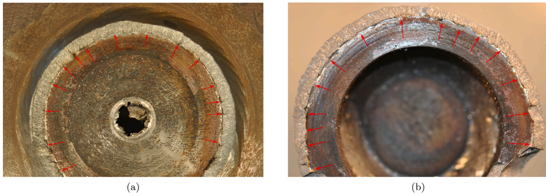
Fig. 7. Fractured surfaces from bending loading: plate view (a) and pipe view (b); some of the crack starting locations have been highlighted by red arrows.
