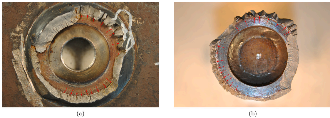
Fig. 8. Fractured surfaces from torsional loading: plate view (a) and pipe view (b); some of the crack starting locations have been highlighted by red arrows.
